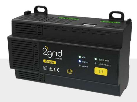
Supervision system for electrical lines and substation condition monitoring. It primarily measures the following parameters:
