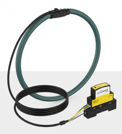
DIN Flex is an active clamp with a converter designed for installation on a DIN rail. This converter transforms the typical millivolt output from Rogowski coils into a standard /1A signal, compatible with measurement and protection devices.
