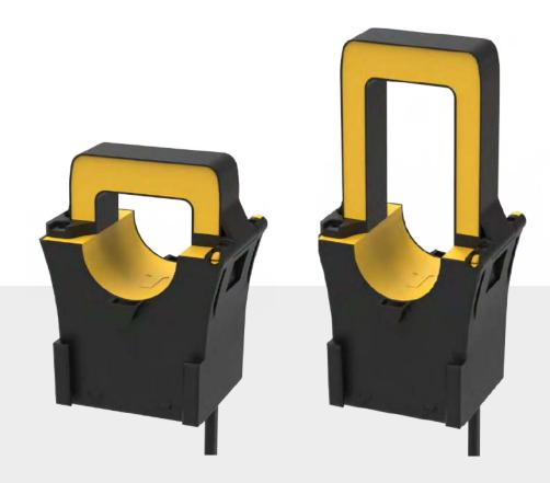
STP split-core transformer series covers a primary current range from 100 to 1000 A, depending on the model, and offers secondary outputs of 1A or 5A. The STP 24 and STP 40 models have an internal circular window with diameters of 24 mm and 40 mm, respectively, while the STP 40L model features a rectangular window of  $40 \times 80$  mm.
