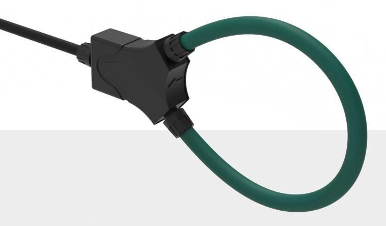
AMS Flex features the smallest detection window in its category, making it the ideal option for OEM companies. This advanced active flexible current transducer perfectly integrates the Rogowski coil with a built-in signal processor, ensuring precise current measurement in various electrical applications.
