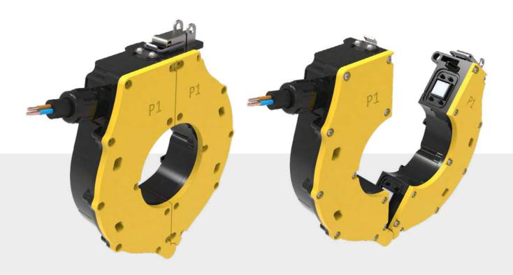
Loop split-core transformers, featuring a circular design and internal window, allow installation on cables up to 55, 80, or 105 mm in diameter without interrupting the primary circuit, saving both time and costs.
